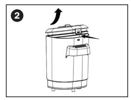
Unscrew the dirty water tank cover & remove the buoy bracket.
