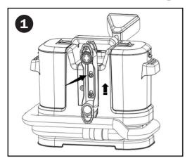
Insert the winding hook into the cylinder of the machine body and push it downward until you hear a "click!" sound, then the installation is complete.
