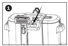
Plug in the appliance. Uncoil the hose from the machine. Press and hold the power button of the main unit, and the machine will sound.
