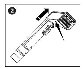
To remove the brush head press and hold the unlock button. When you feel it is released, pull it out to remove the brush head.
