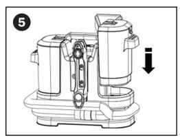
· Reinstall the dirty water tank vertically.
