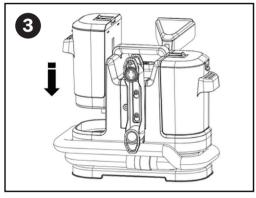
· Reinstall the clean water tank vertically.
