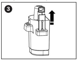
• Remove the buoy bracket & clean the dirty water tank & dry.
