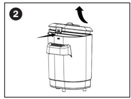
Pull up the latch to open the clean water tank cover. Add the appropriate amount of water. Relock the cover.
