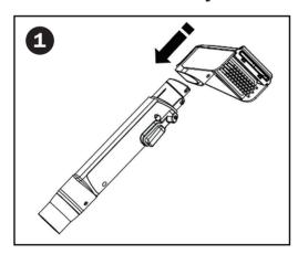
Insert the brush head into position, and when you hear a "click!" the installation is complete.
