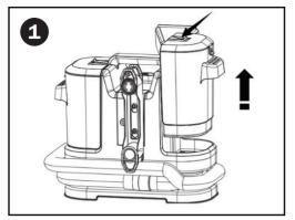
Unplug the appliance. Slide the outer water tank lock hook and remove the dirty water tank vertically.
