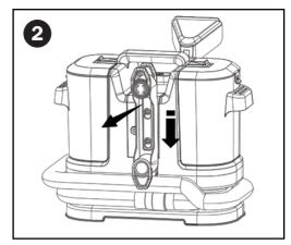
To disassemble the thread winding hook, simply push it up, unhook it, and remove it
