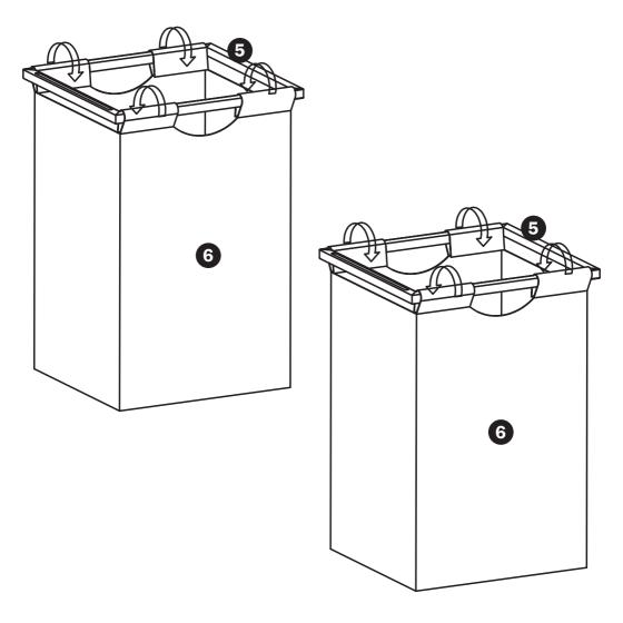
1. Attach the two fabric bags (Part 6) to the two bag frames (Part 5) by folding over the fabric straps and securing.
