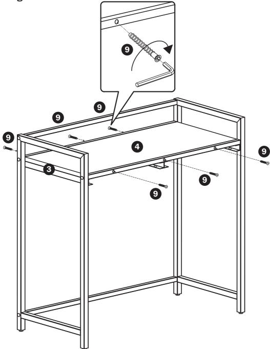
1. Attach the top panel (Part 4) to the top frame (Part 3). Use the Allen key included (Part 11) and 6x 48 mm screws (Part 9). Apply light pressure to the screws but do not tighten them completely.
