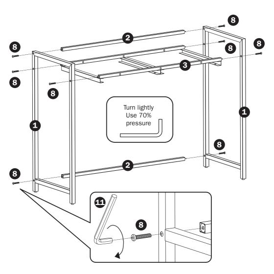
1. Attach the two sides of the laundry basket (Part 1) to the top frame and the two poles (Part 2 and 3). Use the Allen key included (Part 11) and 8x 35mm screws (Part 8), apply light pressure, and do not tighten fully.
